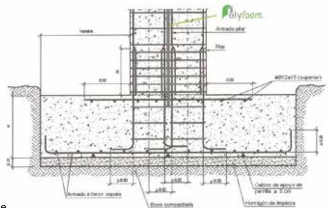
Prevent potential destructive force of concrete, producing damage to himself, we must provide a wide board of intervals that are sealed with Polyfoam®.
